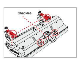
For transport on, for example, a trailer, the machine can be raised. Only use the designated points for attaching the lifting device. The machine must be securely positioned.
