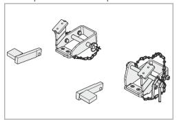
Mounting for carrier vehicles in front mounting with PTO shaft:
