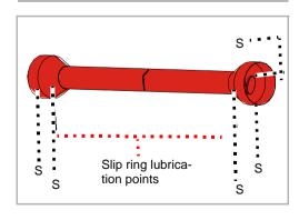
In case of heavy usage or in extreme operating conditions, such as a very dusty environment, more frequent lubrication is required.
