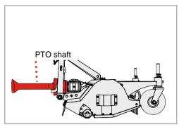
Disconnect the PTO shaft from the carrier vehicle.
