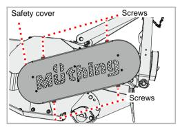
The V-belt is tensioned by a counterweight. If the V-belt is not sufficiently tensioned, it must be retensioned. If there are any tears or the V-belt is damaged, it must be replaced.
