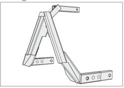
Standard implement triangle for attachment of front-mounted implement to carrier vehicles with tractor triangle with the following category:
