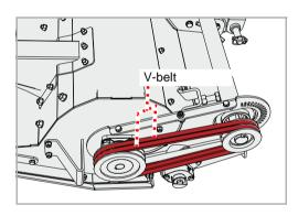
The V-belt unit consists of two narrow V-belts.
