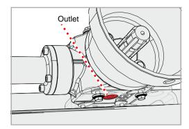
▶ Place a collection container under the outlet for the waste oil
