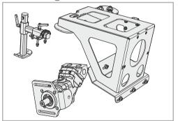
Attachment kit for attachment of front-mounted implement to carrier vehicles. The use of the mounting set is only allowed for machines with hydraulic drive
