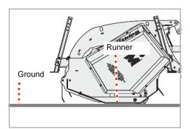
Adjust the height of the lower links via the tractor's three-point linkage so that the machine's runner is parallel to the ground.
