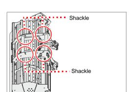
For transport on, for example, a trailer, the machine can be raised. Only use the designated points for attaching the lifting device. The machine must be securely positioned.
