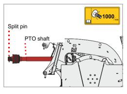
▶ Connect the PTO shaft to the PTO stub shaft of the tractor and ensure that the cotter pin is locked in place on the PTO shaft
