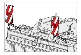
Warning signs with lighting equipment are available for the safety and visibility of the machine in road traffic.
