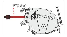
▶ Disconnect the PTO shaft from the tractor
