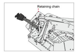
▶ Place the PTO shaft in the retaining chain
